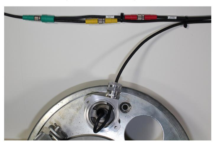
Apply <u>supplied</u> grease to all harness junctions before connecting. Connect the Harness Sensor Junctions together using the Harness Extensions (Straight lengths of cable with red & green connectors on the ends). Match the green end of each Harness Sensor Junction to the green end of each Harness Extension. Match the red end of each Harness Sensor Junction to
