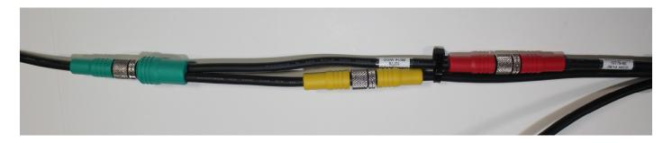
The last yellow sensor connector will attach to the green connector of the last Harness Extension. If the last two manholes are close enough, a final Harness Extension might not be required. In that case, the last yellow sensor connector will attach to the red connector of the last Harness Sensor Junction.
