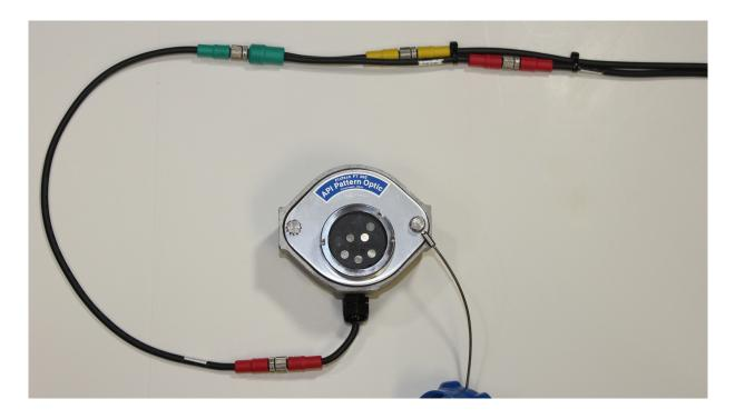
If two sockets are to be connected, use the optional 'Y' Splitter to connect the second socket.
