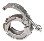
**Clever Clamp with** Service Service Tube Pressure Pressure Α В С 304 Stainless Steel self-locking pin **O.D**. Rating PSI @ Rating PSI @ (in) (in) (in) Part # 304 Stainless Steel 70°F (21°C)<sup>1</sup> 250°F (121°C)1 Part # 1-1/2" 500 300 2.14 1.10 3.04 13SCC-100150 13SCC-100150L 2" 450 250 13SCC-200 13SCC-200L 2.65 1.10 3.53 3" 13SCC-300 350 175 3.72 1.10 4.59 13SCC-300L
