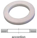
NOTE: The torque (force) required to close the handles on a pair of cam & groove fittings will vary according to the gasket chosen. Due to the nature of the PTFE material, the various PTFE gasket designs will require the most torque, increasing as you go from envelope to encapsulated, and finally, accordion.
