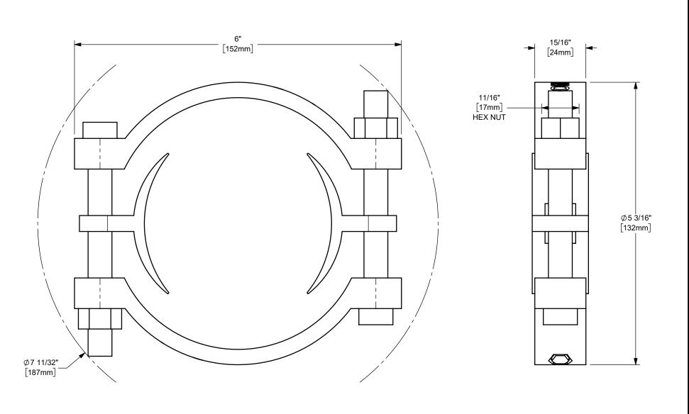
HOSE OD RANGE: 4 2/64" [102.4mm] - 4 18/64" [108.7mm] TORQUE: 40 ft. lbs. [54Nm]
