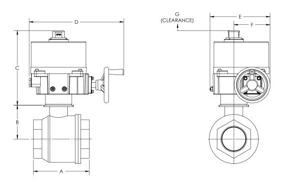
NOTE: Electric actuator shown is OM-3 series. For more information on actuation accessories, see relevant EPRG for electric actuators.
