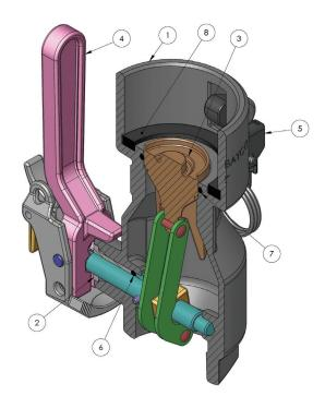
D2CXY-### X = coupling material Y = seal material ### = thread size example part#: D2C72-200 description: D2C stainless steel actuator style coupler with FKM seals and 2" NPT
