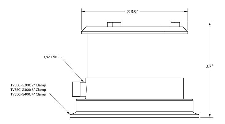
TVSEC-Series Stainless Steel Air and Vacuum Relief Tank Vent Valve - Repair Kits
