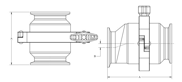
HSC/EHSC-Series Spring Check Valve - Dimensions
