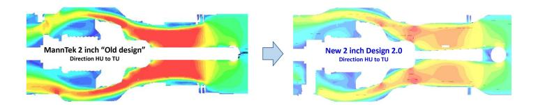
With Design 2.0 both flow capacity and user ergonomics have been improved to a new state-of-the-art level. The flow capacity is increased above 40% through design optimization and has been verified in several incremental flow rate simulations. Design 2.0 offers more optional feature combinations like sensors, locking device, stop before disconnect etc.
