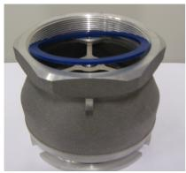
Assemble a new flat sealing (pos.12).
