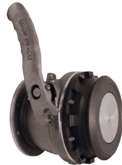
API adapter with fixed handle (poppet can open with API coupler engagement or by using the handle) 5204NG
