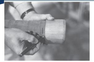
Slide the ferrule all the way onto the hose. Place a mark on the hose at the end of the ferrule. Move the ferrule ½" from the mark just made towards the end of the hose. Place a second mark on the hose at the end of the ferrule.
