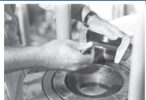
Lubricate the I.D. of both die halves with  ${\sf Crisco}^{\it @}$  (recommended) or high viscosity oil or heavy duty grease.
