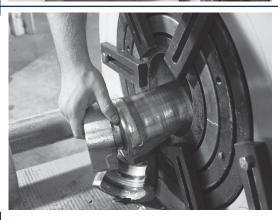
Secure the die holders with tie down bars to prevent the die holders from slipping out of the die bed unexpectedly.
