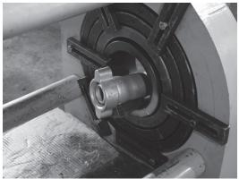
Position a rubber sheet or pad under the die bed. Slowly slide the hose towards the pusher. When the die clears the die holder, one or both halves may fall to the floor. If one half remains on the ferrule, tap it with a mallet until it releases. If both halves remain on the ferrule, it may require the halves be pried apart at the seam.
