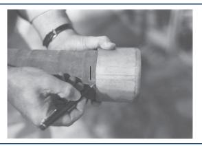
Hold the ferrule against the stem collar (sizes  $1\frac{1}{2}$ " - 3" only). Using a small ruler or other measuring devise, insert it between the stem and ferrule until it contacts the stem collar. Measure the depth at the end of the ferrule. Place a mark on the hose (the hose end to be assembled) that corresponds with this measurement.
