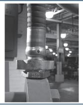
Wipe excess lubricant from hose and ferrule. Bring hose with stem and ferrule back through die bed.
