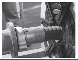
Move the directional control lever to the "REVERSE" position and depress the button on the remote. Retract the cylinder until there is sufficient room for the stem and ferrule to clear the die bed.
