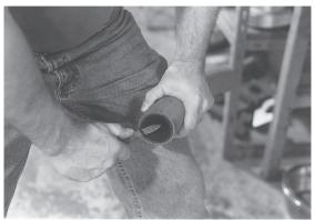
Assuring that the hose end is cut square, chamfer the I.D. of the hose  $\frac{1}{6}$ " at a 45° angle. This will aid in stem insertion. If the hose is to be static grounded, follow hose manufacturers procedure for proper static grounding.
