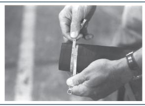
Accurately measure the hose O.D. with a diameter tape. Each end of the hose should be measured to guarantee the correct ferrule and die selection. Select the correct ferrule and die based upon the hose free O.D. just measured from the chart.
