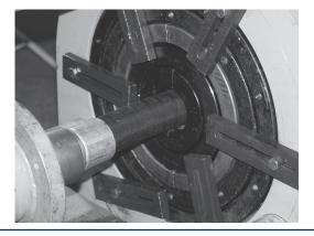
While holding the die in place with one hand, place one of the tie down bars over the die so that it does not come out of the die holder unexpectedly. Secure the tie down bar by tightening the holt
