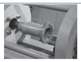
Install the 6" Main Pusher (MPUSH600) by sliding it onto the rod cap of the ram cylinder. Make sure that the pusher is all the way on the rod cap. Install the appropriate adapter pusher (by coupling size) into the main pusher.
