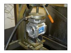
When the leakage test is made without leakage, the ball valve is blown dry and clean with air and is ready for use again.
