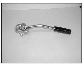
Mount the handle into the spindle, make sure that the hole for the stop pin is open
