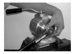
Screw on one of the end covers, tighten until the end cover comes in it's right position with the body
