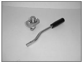
Remove the handle from the spindle
