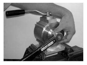
Screw on the other end cover with the assembly tool, tighten both sides until they are equally recessed.
