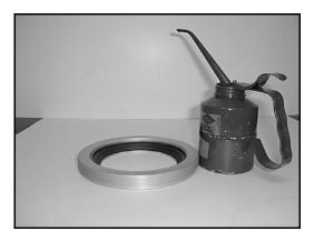
Use grease on the black Teflon packing and the threads on the both end covers
