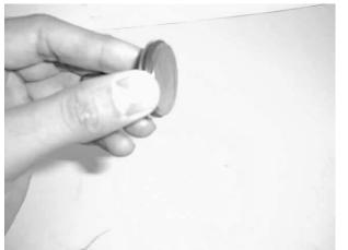
Change the O-ring on the piston to a new greased O-ring.
