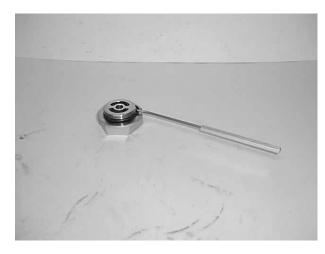
Change the O-ring on the threaded part to a new one. Use a greased O-ring.
