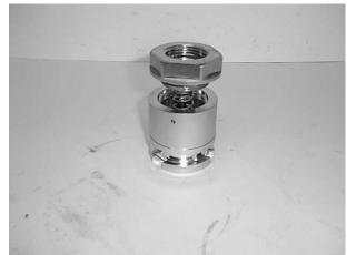
Remove the flat sealing. NPT-thread does not have a flat sealing.
